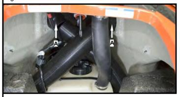
Loosen clamp (A) and remove fuel filler hose from tank.
