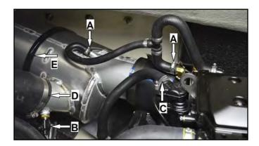
At exhaust clamp loosen t-bolt nut enough to allow end ('T') to be removed from band clamp. Remove exhaust clamp. (Figure EX3)
