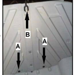
Remove darts (A) and remove vent hoses from hull. (Figure 4)
