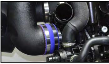
Reattach cable to exhaust temperature sensor. If using OEM breather system install formed hose onto crankcase vent valve and barbed fitting previously installed into Inlet Tube A. Short end of formed hose goes onto barbed fitting.
