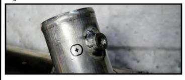
Hole center should be at 3:00 to 4:00 position with respect to index notch in waterbox tube. (see figure EX1)
