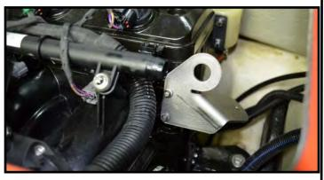
Loosen bolts in supplied threaded ring and slip over supercharger inlet. Note: Assemble ring so that both ring halves have two dots showing. (This will align threads in both halves.) Position threaded ring against flare on supercharger inlet and tighten allen screws. **Do not over tighten screws. Do not use Loctite on threads.** (Figure 13)
