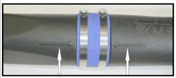
While maintaining alignment tighten hose clamps on coupler between A and B. **Do not over tighten clamps.**
