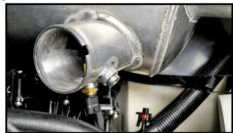
Reinstall waterbox and coupler assembly onto exhaust manifold reversing removal procedure. **NOTE:** Do not tighten hose clamp yet. Tip: Lubricate inside of coupler and outside of exhaust manifold with glass cleaner to ease installation.
