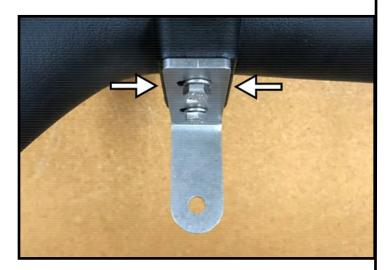
NOTE: Bracket is slotted to accommodate superchargers with spacer plates.
