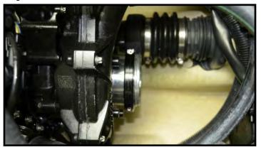
Screw velocity stack onto threaded ring. Tighten hand tight. Be sure velocity stack is seated all the way onto threaded ring. (Figure 14)
