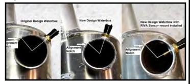
Note that the location of the temperature sensor is changed in relation to the index notch on the waterbox outlet. The new location of the temperature sensor interferes with Inlet Tube A of this kit. If your ski is equipped with one of these waterboxes the sensor must be relocated to install this kit.
