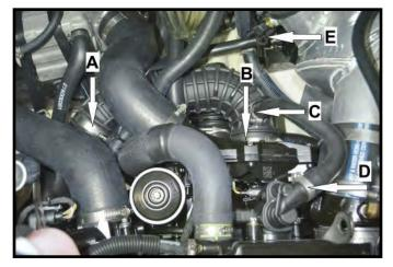
Sea-Doo changed the location of the temperature sensor in the waterbox during production of 2016 model 300s. (Figure EX1).
