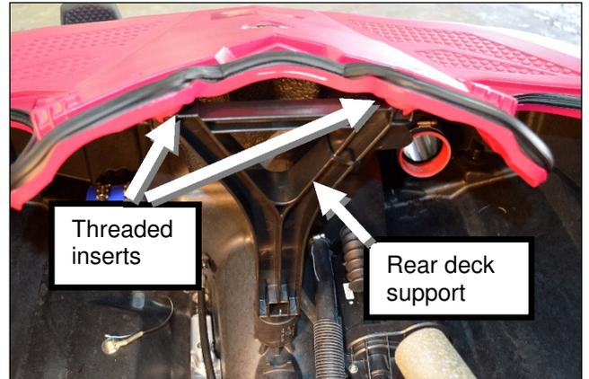
Guide steering cable through cable access hole on top deck. Use care to ensure the rubber deck seals are properly sealing. Line up screw holes between the top & lower deck.
