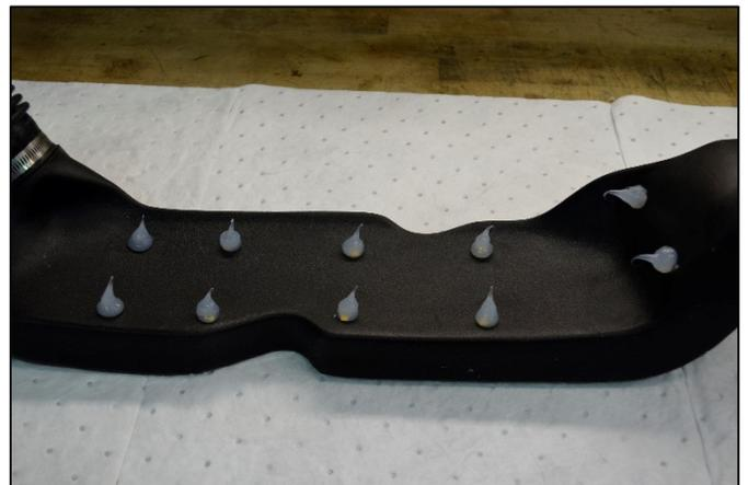
Step 17: Immediately after applying the sealer, and before it cures, place the assembled Power Filter Unit in location and press it against the side of the fuel tank as shown in the photo.
