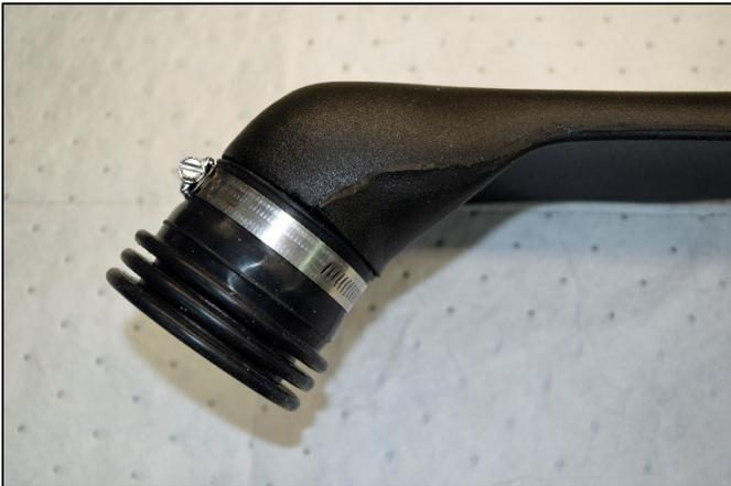
Step 15: Thoroughly clean the mounting surface of the supplied Air Intake Duct with a non-residual cleaner and install the supplied Flame Arrestor and hose clamp onto the Air Intake Duct and tighten the clamp. The Flame Arrestor flange has a stop inside and it should be pushed on until it is fully seated. Do not overtighten the clamp!
