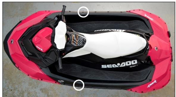
Step 22: Install rear support screws (circled in illustration below) Torque to 5.5 N.m / 49 inch lbs.
