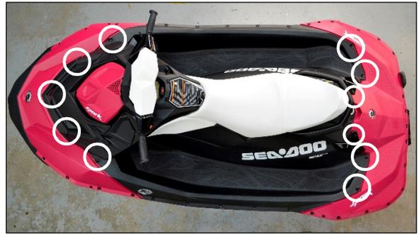
Step 25: Reinstall self tapping screws (3) at gas fill cap. Torque to 4.5 N.m / 40 inch lbs. (refer to step 10)
