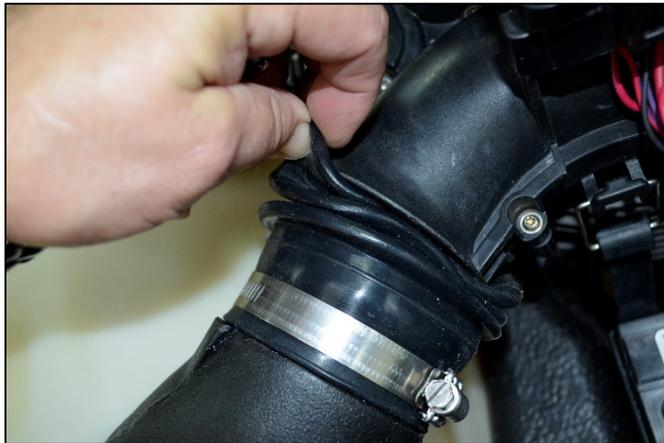
The flange of the factory air box inlet should seat in the second fold of the Bellows Coupler.
