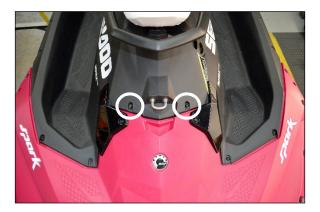
Step 23: Install side rail bolts, nuts & washers. (circled in illustration below) Torque to 3.5 N.m / 31 inch lbs.
