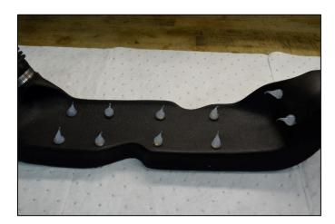
Step 17: Immediately after applying the sealer, and before it cures, place the assembled Power Filter Unit in location and press it against the side of the fuel tank as shown in the photo.
