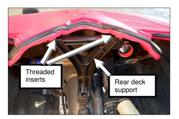
Guide steering cable through cable access hole on top deck. Use care to ensure the rubber deck seals are properly sealing. Line up screw holes between the top & lower deck.
