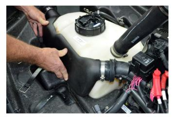
Step 18: Reconnect the fuel tank hold down straps and the fuel pump electrical connector.
