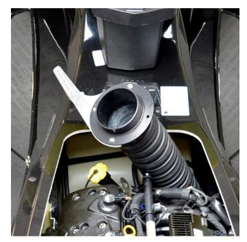
Install supplied Power Filter with supplied pre-filter onto opposite side of support flange. **NOTE: Do not over tighten clamp.**
