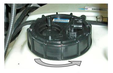
Raise fuel pump out of fuel in tank. **DO NOT REMOVE COMPLETELY.** Tilt forward to drain excess fuel.
