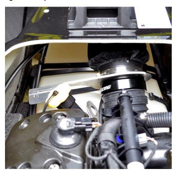
Secure Power Filter/Duct Support to hull. **NOTE: Apply red Loctite to threads. Do not over tighten bolts.**
