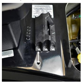
Using a square measure 1-7/8" straight out (to left side) from edge of seat bracket.
