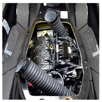
Install supplied billet band clamps onto ends of ducting. **NOTE:** Inside of clamps are threaded. Twist onto ducting until edge is flush with end of ducting. **TIP:** Spray glass cleaner onto outside of ducting to ease installation.
