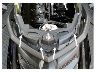
Remove bolts (1 at rear) and reusable clips (4 at front) securing decorative cover to outside of grab handle.
