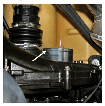
Lubricate inside of black plastic velocity stack and outside of supercharger inlet with glass cleaner. Push black plastic velocity stack firmly onto supercharger inlet until fully seated.
