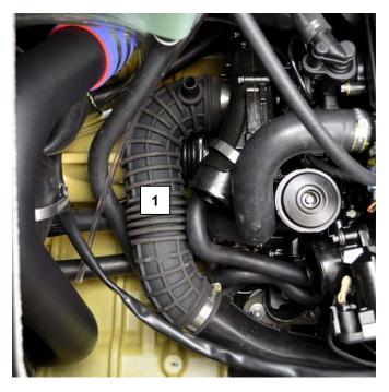
At front right side of engine loosen clamp securing plastic air intake runner to air box.
