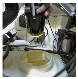
NOTE: Place a shop rag on top of tank and over top of fuel pump to prevent fuel spill.
