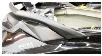
Remove coolant overflow reservoir. Remove grab handle (6 bolts).
