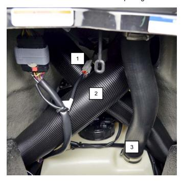
Disconnect fuel supply hose<sup>1</sup> and fuel pump electrical connector<sup>2</sup>.
