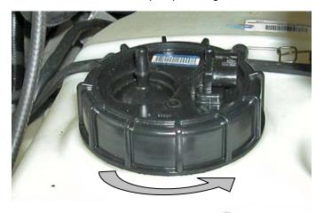
Raise fuel pump out of fuel in tank. **DO NOT REMOVE COMPLETELY.** Tilt forward to drain excess fuel.
