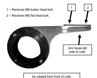
Test fit supplied Power Filter/Duct Support Bracket using supplied hardware. Bracket mounts inside hull under seat bracket.
