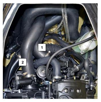
Remove and discard hose between engine breather and stock air intake tubing. Retain hose clamps.
