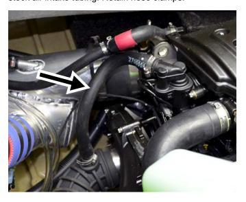
Install RIVA Oil Catch Can/Engine Breather Kit (part# RS19050-BCC).
