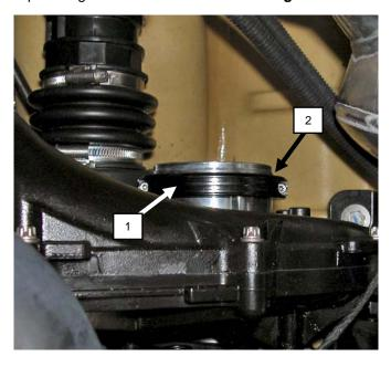
Install supplied tapered plastic flange onto billet adapter flange. **NOTE:** Plastic flange and billet adapter are threaded. Do not over tighten.
