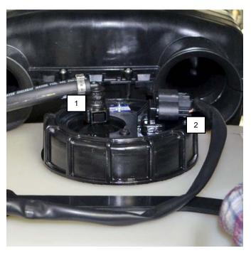
NOTE: Fuel system is pressurized. Cover fuel supply hose connector with a shop rag to prevent fuel spill.
