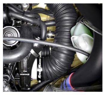
Reconnect hoses to supercharger outlet and throttle body inlet. **NOTE: Do not over tighten clamps.**
