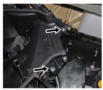
Inside air intake silencer squeeze outlet hose together. Remove air intake silencer by lifting up. Discard.
