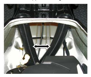
**NOTE:** Each tube has one pin securing tube to inlet at opening in hull.
