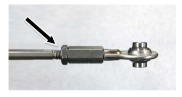
Replace steering cable in reverse order of removal. **NOTE: Do not over tighten bolts.**
