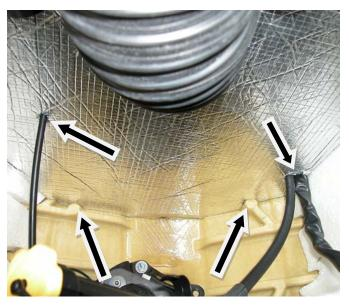
Feed steering cable through small hole at left side of thermal bulkhead.
