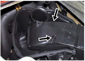
Remove bolts (2) securing air intake silencer to motor.
