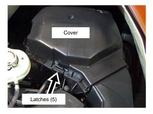
Lift cover and pull forward to gain access to blow-by hose. Remove hose. Discard lid.
