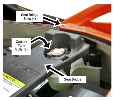
Remove seat bridge from hull and set aside. Take care not to allow engine coolant tank to tip over during installation process.
