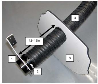
Spray glass cleaner on outside of ducting and in large opening at center of thermal bulkhead. Insert ducting through opening on silver side until 12~13in of ducting extends beyond white side of thermal bulkhead. **TIP:** Twist ducting as you push it through bulkhead.
