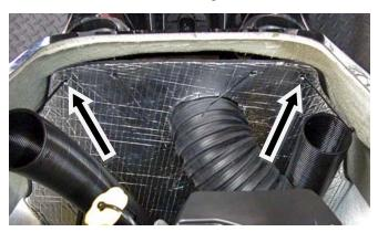
Place top edge of thermal bulkhead forward of engine compartment air inlets by carefully bending top of thermal bulkhead back towards engine. Once in place thermal bulkhead will be rest in place vertically.
