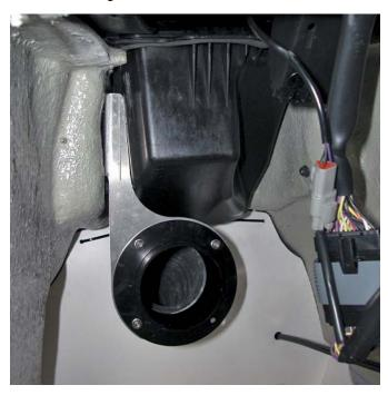
**NOTE:** Filter/Duct Support is threaded. Apply red Loctite to screws. Do not over tighten.
