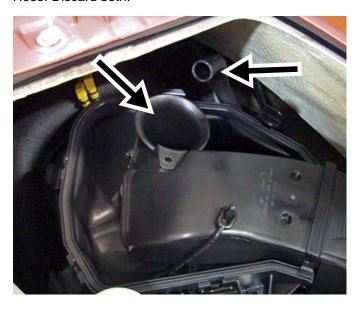
Remove rubber straps (3) securing air intake tube. Remove air intake tube and discard.
