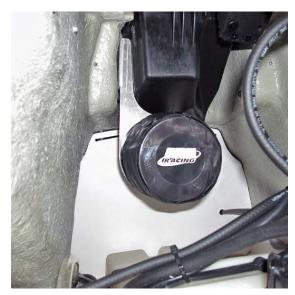
Replace steering cable adjustment nut. **NOTE:** Make sure nut is adjusted to same distance as before it was removed.
