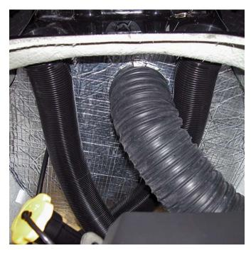
Feed long end of ducting into hull at front of engine; along right side of craft; under intake manifold; around back of engine. Pull open end of ducting past intake manifold and up out of engine compartment.
