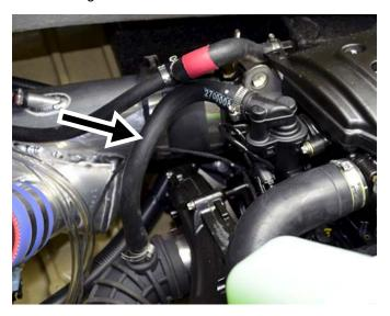
Remove supercharger air inlet hose and discard.
