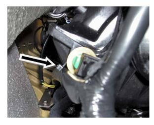
Remove flat head screws (2) from Filter/Duct Support. Place end of ducting with Filter/Duct Support into engine compartment and rest on top of fuel tank.
