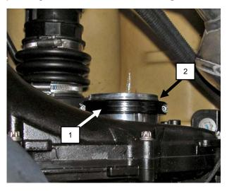
Install supplied tapered plastic flange onto billet adapter flange. **NOTE:** Plastic flange and billet adapter are threaded. Do not over tighten.
