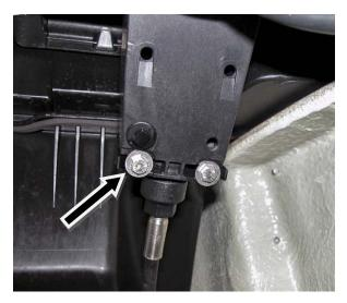
Lift steering cable up and away from support to remove locking collar.
