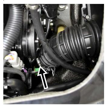
Remove plastic air intake runner through rear of engine compartment and discard.
