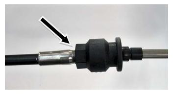
Replace steering cable end. **NOTE:** Make sure jam nut is set to same distance as before it was removed. Check alignment with steering arm to prevent binding.
