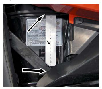
**NOTE:** Align template vertically with bolt for seat bracket hinge. Top of template is placed flush against edge where hull and glove box meet.
