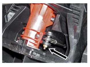
Inside hull under steering column locate steering cable support arm. Cut zip tie securing electrical wiring.
