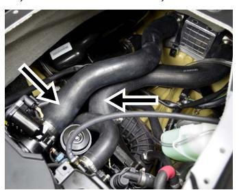
Remove hose between engine breather and stock air intake tubing.
