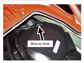
Remove air intake silencer baffle (pull up) and Blow-by Hose. Discard both.
