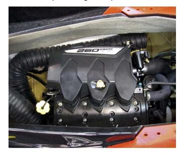
Install supplied billet band clamp onto end of ducting. **NOTE:** Inside of clamp is threaded. Twist onto ducting until edge is flush with end of ducting. **TIP:** Spray glass cleaner onto outside of ducting to ease installation.
