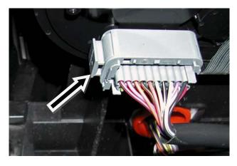
Remove gauge support by unclipping locking tabs on each side (2 outside/2 inside) and set aside.
