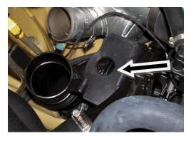
Remove supercharger inlet hose (1 clamp) and discard.
