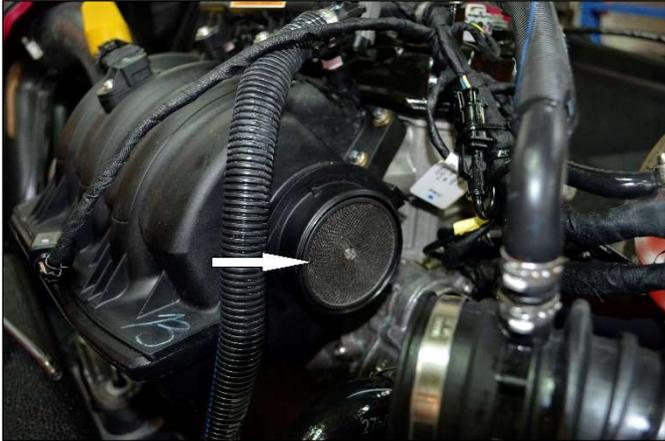
Step 14: Remove the flame arrestor ribbon by inserting the blade of a thin bladed straight screwdriver between the manifold inlet sidewall and the ribbon and prying gently outward. Proceed slowly working at several points around the circumference of the ribbon taking care not to damage the manifold or the rubber ring around the ribbon.
