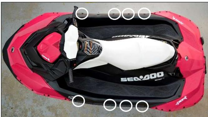
Step 22: Reinstall rear trim pieces (refer to step 8) & reinstall self tapping screws at front & back of hull. (circled in illustration below) Torque to 5.5 N.m / 49 inch lbs.
