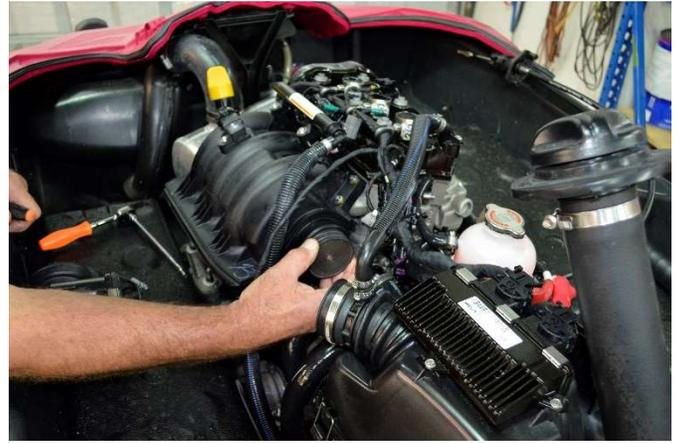
Step 15: remove the rubber holder from around the flame arrestor ribbon.
