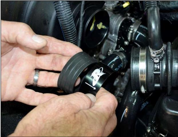
Step16: Slip included stainless oetiker clamp onto the rubber flange at the intake manifold end of the throttle body. Slide the rubber flange over the intake manifold inlet. Note the locating stud shown in the photo below and make sure it aligns with the cutout in the rubber flange as shown. Use the Oetiker Pincer Tool to secure the clamp.
