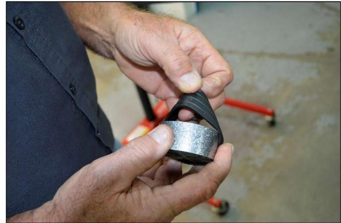
Step 15: Before installing the rubber holder onto the billet sleeve note the direction of the arrow on the sleeve. When assembled this arrow must point toward the throttle body.
