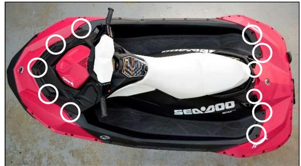
Step 23: Reinstall self tapping screws (3) at gas fill cap. Torque to 4.5 N.m / 40 inch lbs. (refer to step 10)
