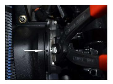
Step 17: Slide the original hose clamp onto the airbox hose pushing it well up onto the hose. Slip the hose onto the throttle body. Place the hose clamp into position and tighten. Do not over tighten.
