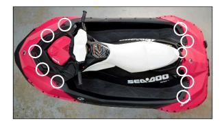
Step 23: Reinstall self tapping screws (3) at gas fill cap. Torque to 4.5 N.m / 40 inch lbs. (refer to step 10)
