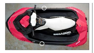
Step 20: Install rear support screws (circled in illustration below) Torque to 5.5 N.m / 49 inch lbs.
