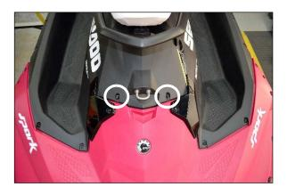
Step 21: Install side rail bolts, nuts & washers. (circled in illustration below) Torque to 3.5 N.m / 31 inch lbs.
