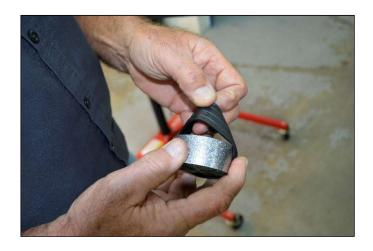
Step 15: Before installing the rubber holder onto the billet sleeve note the direction of the arrow on the sleeve. When assembled this arrow <u>must</u> point toward the throttle body.
