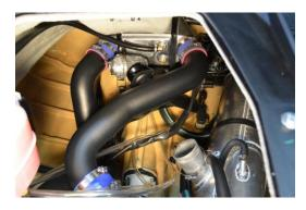
Reconnect the waterbox to the exhaust outlet using the original exhaust hose, RIVA Free Flow tube, or RIVA
