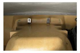
Locate the pump mounting studs inside the hull.(see illustration below) Remove the 13mm nut, but leave the washer in place. Slide the supplied straight strap hook over each stud. Slide the supplied 8mm washer over each stud. Install strap hook so the clip is on top & facing out. (see illustration below) Reinstall the 13mm nut & torque to 18 ft. lbs.
