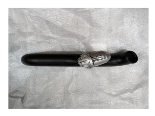
Install supercharger to intercooler tube. Adjust couplers & secure with supplied clamps. **NOTE: Do not over tighten clamps.**
