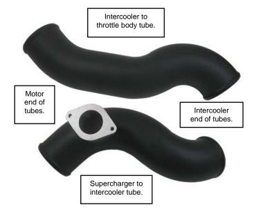
Install one supplied silicone coupler completely onto motor end of intercooler to throttle body tube. **TIP:** Apply a generous amount of glass cleaner to aluminum tube and inside of coupler. Install tube between intercooler and throttle body. Secure hose clamp at intercooler side of tube. Slide opposite coupler onto throttle body inlet and secure clamps.
