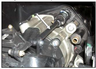
Inside hull remove VTS from thru-hull fitting and set aside.
