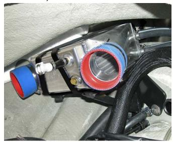
Route loose end of Line 1 towards water inlet fitting at pump transom. Install and secure using OEM hose clamp. Route loose end of Line 2 towards left side of engine, then forward and connect to barbed fitting at underside of front of exhaust manifold. Secure using OEM hose clamp. NOTE: Be careful not to kink hoses. It may be necessary to trim excess hose for proper fit. Do not over tighten clamps.
