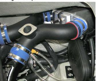
Install recommended **RIVA Blow-off Valve Kit** onto supercharger to intercooler tube using instructions supplied with B.O.V. kit.
