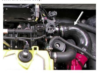
**NOTE:** If using a RIVA Blow-off Valve Kit, remove completely (including vacuum line). A longer vacuum line or vacuum cap is supplied with this kit.
