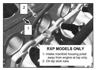
RXP ONLY. RXT & GTX-SC Proceed to next paragraph. NOTE: Do not remove completely. Do not lift or pull upward. Take care not to dislodge oil dipstick tube from crank case.
