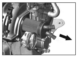
RXP ONLY. RXT & GTX-SC Proceed to next paragraph. Allow intake manifold housing to relax against engine. Replace Torx® screws (7) previously removed and torque to 6 N•m (53 lbf•in). NOTE: Use blue Loctite. Do not replace ignition coils and ECU connectors if you plan to install a Blow-off Valve.
