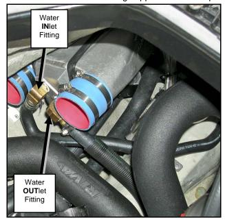
Route loose end towards water inlet fitting at pump transom and secure using supplied hose clamp.
