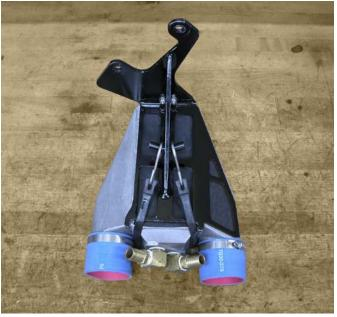
Apply silicone sealant to surface area of mounting bracket that will be placed against hull. Install and secure Power Cooler/Mounting Bracket assembly using stock hardware. NOTE: Apply red Loctite to bolts. Torque to 61 N•m (45 ft•lb).
