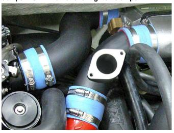
At this point you are left with installing your option for the mounting flange on the supercharger discharge tube. RIVA Racing strongly recommends the use of a Blow-off Valve to prevent unnecessary wear on the supercharger clutch. We offer the following options:
