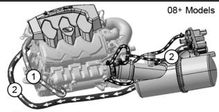
Disconnect Line 1 at front of exhaust manifold and remove completely. Disconnect Line 2 at pump transom and remove completely. **NOTE:** Retain both lines for use when installing supplied intercooler.
