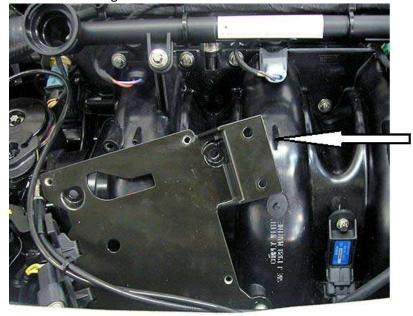
Drill through this fitting into manifold and attach hose.
