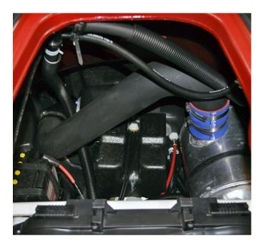
Insert curved end of Free Flow Exhaust Tube into coupler on water box outlet. **TIP:** Use window cleaner to ease installation. **NOTE:** It may be necessary to rotate water box to align Free Flow Tube with exhaust outlet coupler. To do so loosen hose clamp securing exhaust coupler to water box.
