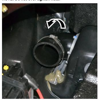
NOTE: Do not use any sealant when replacing exhaust outlet. Only nuts and washers should be on outside of hull after replacing exhaust outlet.
