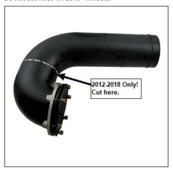
Thoroughly clean inside of OE exhaust outlet hose and outside of water box outlet with a non-residual cleaner.
