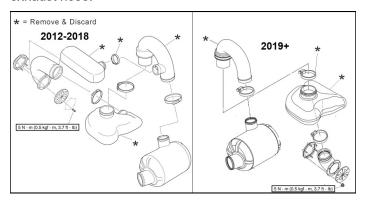
Loosen hose clamp securing OE exhaust hose to the water box (muffler). Disconnect hose from water box.
