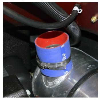
Loosely place one OE clamp over modified exhaust outlet hose and water box coupler.
