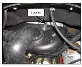
2019+ Loosen clamp under left rear of resonator and remove resonator with exhaust hose.
