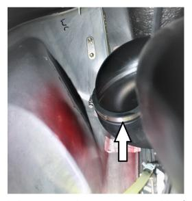
In jet pump area locate and remove rubber flap to right of jet pump unit.
