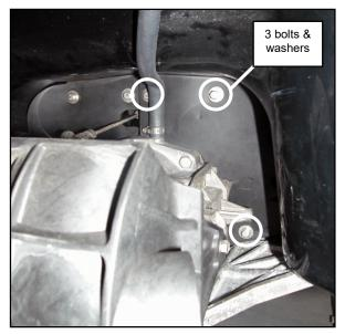
At exhaust outlet remove the six nuts and washers securing exhaust outlet to hull. **Note position exhaust outlet hose is facing prior to removing.**
