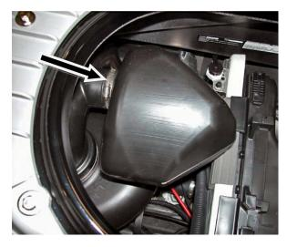
Remove exhaust hose (2 clamps). Leave clamp at water box outlet.
