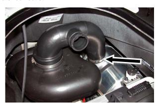
Remove exhaust baffle (1 clamp). Retain clamp.
