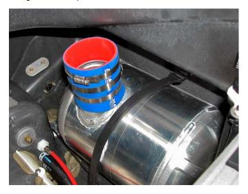
Place one stock clamp and one supplied clamp onto coupler.
