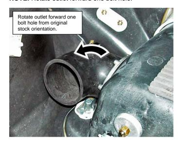
Secure outlet using stock nuts and washers. **NOTE: Do not over tighten nuts.**
