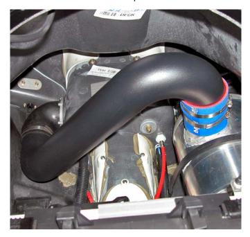
**NOTE:** It may be necessary to rotate water box to align outlet with Free Flow Tube. Loosen clamp securing coupler at water box inlet.
