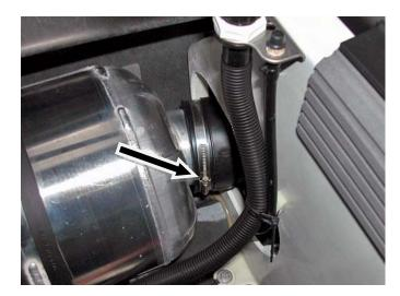
Slide one of the loose clamps on water box coupler over tube to exhaust outlet and secure. **NOTE: Do not over tighten clamp.**
