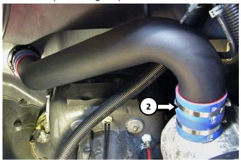
Remove coupler and exhaust tube from waterbox outlet.
