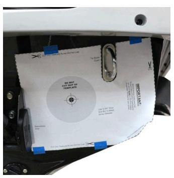
Using a 3-3/4" hole saw bit remove section with gray circle.
