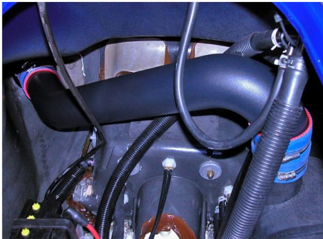
Tighten hose clamps (2) securing Exhaust Tube in place. **NOTE: Do not over tighten clamps.** Tighten coupler securing exhaust pipe to water box inlet if previously loosened.
