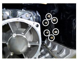
Place supplied billet exhaust outlet block-off onto stock exhaust collar so that raised side of block-off faces the same direction as the six threaded studs. Install supplied rubber gasket over studs and onto billet block-off (adhesive side first).
