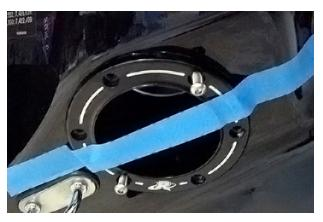
From inside of hull, carefully place supplied billet collar onto exhaust outlet. Ensure raised stand offs are toward the hull.
