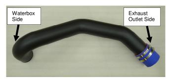
Install exhaust outlet side of tube (side with coupler) onto rear exhaust outlet inside hull. Slide 2nd hose clamp down coupler & into position on outlet. Secure coupler onto outlet with clamp. **Note: Do not over tighten clamp.**
