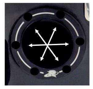
Drill one bolt hole and insert one supplied M6 button head screw. Repeat for remaining five bolts working from opposing sides.
