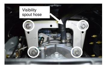
Remove lower reduction nozzle bolts (2). Remove reduction nozzle with reverse gate from jet pump.
