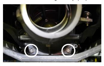
Remove nuts (6) securing stock exhaust outlet to hull. Remove and discard exhaust outlet hose. Retain nuts and exhaust outlet collar.
