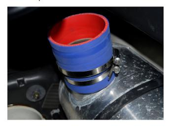
Install supplied coupler onto outlet end of supplied rear exhaust pipe. Secure using supplied hose clamp. **Note: Do not over tighten clamp.**
