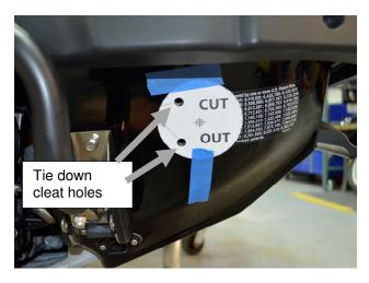
Drill a small pilot hole in the center of the template. (at the cross hairs) Remove template. Using a hole saw bit no larger than 3-3/4", create hole for outlet.
