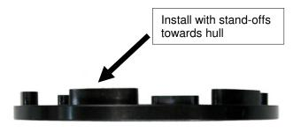
Slide collar onto outlet until you feel it touch the ends of the two bolts. Carefully try to center the top of one or both of the bolts in the threads in the collar. From outside of hull slowly tighten bolt aligned with collar. Once you feel it grab tighten a few turns. Move to opposite bolt and do the same. Once bolts easily screw into collar install remaining bolts and tighten evenly. NOTE: Apply blue Loc-tite to bolts. Do not over tighten.
