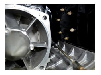
Inside hull at right rear area remove nuts (2) securing tie down cleat. Remove cleat.
