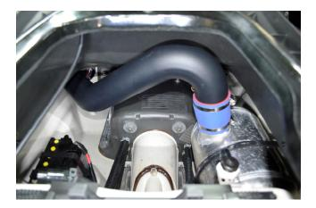
Reinstall reduction nozzle with reverse gate onto jet pump. Secure in position with 2 bottom reduction nozzle bolts. Do not fully tighten bolt yet. **Note: Apply blue Loctite to bolts.**
