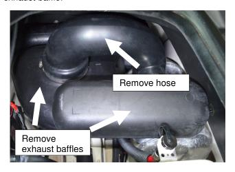
Retain hose clamp on exhaust outlet hose and from waterbox for later use. Remove floatation foam located on top of pump tunnel.
