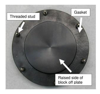
Install stock exhaust outlet block-off from inside hull. Secure using stock nuts (6). **NOTE: Do not over tighten nuts.**
