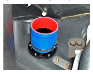
Thoroughly clean outside of water box outlet with a nonresidual cleaner. Install second supplied exhaust coupler onto outlet and secure with clamp left on outlet during removal process. **NOTE: Do not over tighten clamp.** Loosely install two previously removed OE clamps over exhaust coupler.
