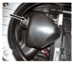
Remove exhaust hose (2 clamps) and discard. Leave one clamp at water box outlet.
