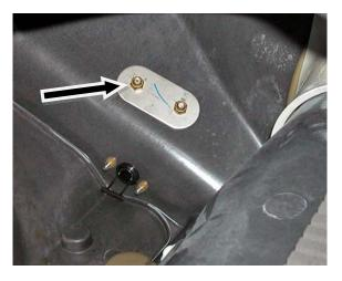
Outside of hull remove tie down cleat. Using a straight edge draw a line 3~4 inches long towards jet pump directly in line with original mounting holes.
