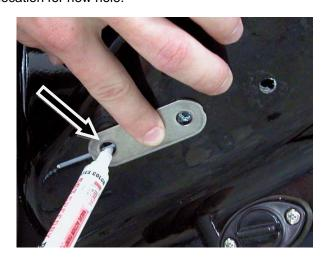
Drill new hole. Replace tie down cleat. **NOTE: Apply** "below waterline" silicone sealant around threaded posts on cleat. Do not over tighten nuts.
