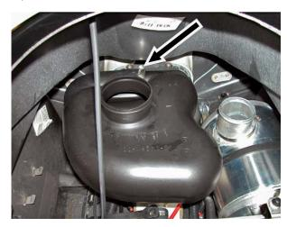
At jet pump remove bolts (2) and nut (1) securing sound suppression flap at right side of pump.
