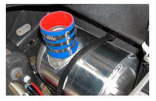
Insert straight end of supplied exhaust tube into rear exhaust outlet coupler. Insert curved end of exhaust tube into coupler on water box outlet. **TIP:** Use window cleaner to ease installation.
