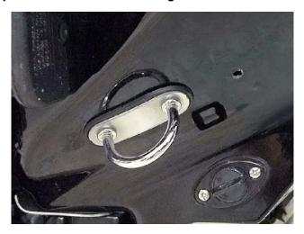
Cut out supplied template (last page) and affix to right rear side of hull using tie down cleat as a reference point.
