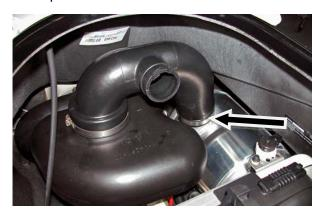
Remove exhaust baffle (1 clamp) and discard. Retain clamp.
