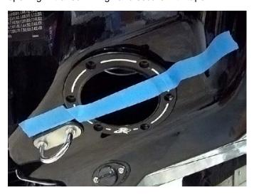
Drill one bolt hole and insert one supplied M6 button head screw. Repeat for remaining five bolts working from opposing sides.
