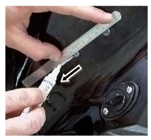
Using exterior tie down cleat mounting plate, mark location for new hole.
