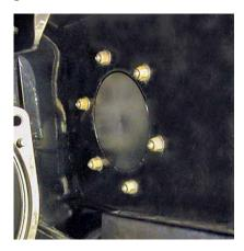
Inside hull at right rear area remove nuts (2) securing tie down cleat.
