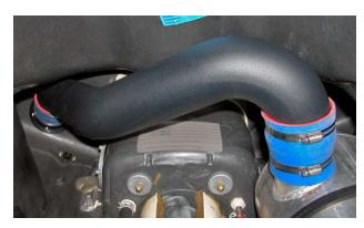
**NOTE:** It may be necessary to rotate water box to align outlet with exhaust tube. Loosen clamp securing coupler at water box inlet.
