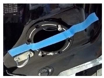
From inside of hull carefully place supplied billet collar (side with raised stand-offs towards hull) onto exhaust outlet.
