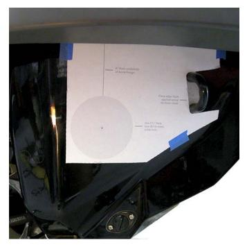
Using a 3-3/4" hole saw bit drill opening for supplied billet exhaust outlet.
