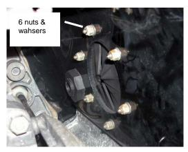
Remove OEM exhaust outlet hose from inside of hull. Remove aluminum ring with studs from exhaust outlet hose. **Retain ring.** Discard exhaust outlet hose and exhaust outlet valve.
