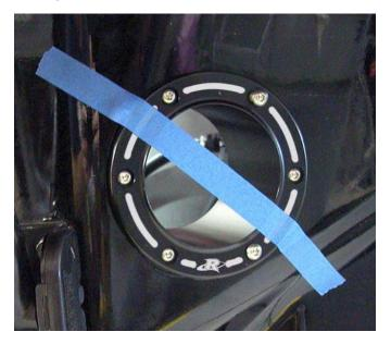
Drill one bolt hole and insert one supplied M6 button head bolts. Repeat for remaining bolts.
