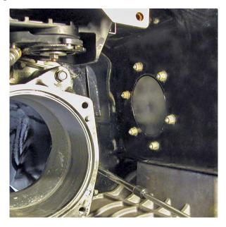
Insert supplied billet exhaust outlet into newly created opening in transom so that 'R' logo is at bottom. Secure with tape.
