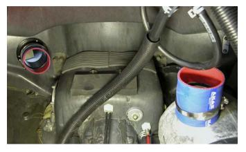
Thoroughly clean outside of water box outlet using a non-residual cleaner. Install second supplied exhaust coupler halfway onto outlet and secure with one of the previously removed OEM hose clamps. **NOTE: Do not over tighten clamp.** Loosely install the last previously removed OEM hose clamp over exhaust coupler.
