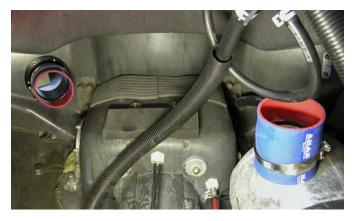
Thoroughly clean outside of water box outlet with a nonresidual cleaner. Install second supplied exhaust coupler halfway onto outlet and secure with one of the previously removed OE hose clamps. **NOTE: Do not over tighten clamp.** Loosely install the last previously removed OE hose clamp over exhaust coupler.
