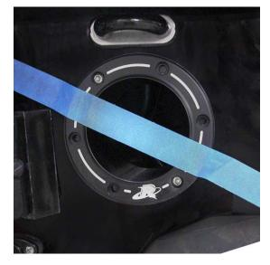
Drill one bolt hole and insert one supplied M6 button head screw. Repeat for remaining five bolts.
