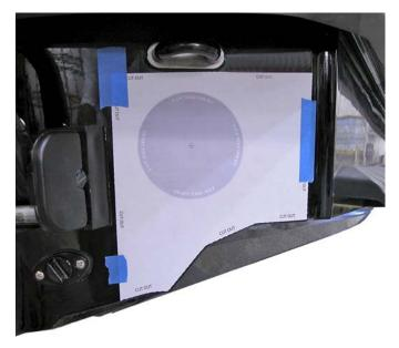
Using a 3-3/4" hole saw bit cut remove section with gray circle.
