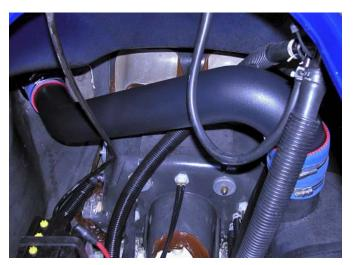
Tighten hose clamps (2) securing Exhaust Tube in place. **NOTE: Do not over tighten clamps.** Tighten coupler securing exhaust pipe to water box inlet if loosened.
