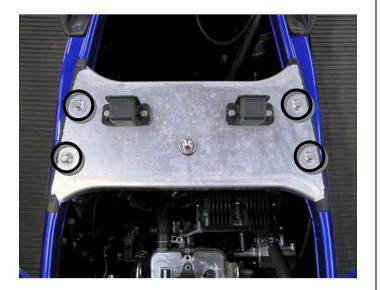
Inside engine compartment at rear of craft remove and discard exhaust baffles<sup>1</sup> and hose<sup>2</sup> between water box and exhaust outlet hose. **Save OE clamps for installation portion.**
