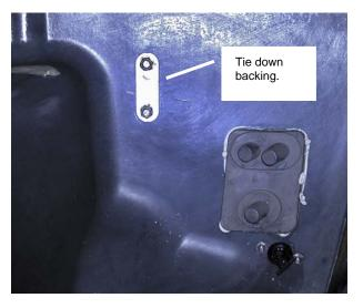
Remove cleat. Separate metal plate from cleat. Usnig a M8 bolt place plate on hull with bolt in upper hole. Swing bottom up to the left so that plate is horizontal. Secure with tape.
