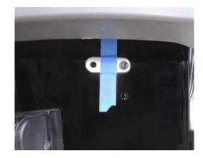
Drill a new hole. Replace metal plate onto cleat. Replace cleat and secure from inside. **NOTE: Do not over tighten nuts.**
