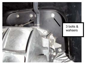
At exhaust outlet remove the six nuts and washers securing exhaust outlet to hull.
