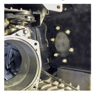
Insert supplied billet exhaust outlet into newly created opening in transom so that 'R' logo is at bottom and contour of flange is flush against hull. Secure with tape.
