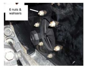
Remove OE exhaust outlet hose from inside of hull. Remove aluminum ring with studs from exhaust outlet hose. **Retain ring.** Discard exhaust outlet hose and exhaust outlet valve.
