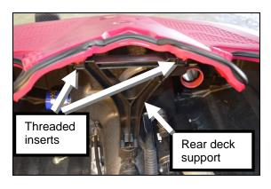
Guide steering cable through cable access hole on top deck. Use care to ensure the rubber deck seals are properly sealing. Line up screw holes between the top & lower deck.
