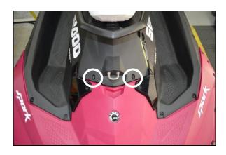
Step 25: Install side rail bolts, nuts & washers. (circled in illustration below) Torque to 3.5 N.m / 31 inch lbs.
