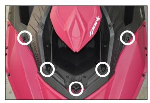
Step 6: Remove the eight (8) circled self tapping screws at the rear of the top deck. Remove rear trim pieces by sliding out of position. (see illustration below)
