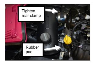
Step 20: **Free Flow Exhaust application:** Install supplied 2.75"x2.25" reduction coupler on waterbox outlet. Spray glass cleaner on inside of coupler to ease installation. Secure coupler on waterbox with supplied hose clamp. **Do not over tighten clamp.**
