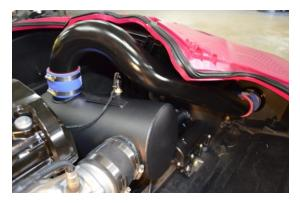
Step 22: Reinstall top deck to lower deck. (refer to step 9) Make sure rear deck support is correctly positioned and top threaded inserts (2) are in place. (see illustration below)
