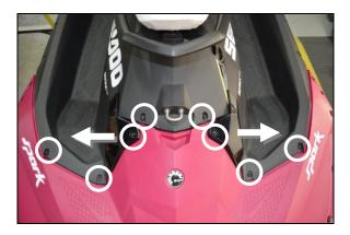
Step 7: Remove the ten (10) circled Torx screws & nuts on the sides of the hull. (see illustration below)
