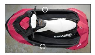
Step 24: Install rear support screws (circled in illustration below) Torque to 5.5 N.m / 49 inch lbs.
