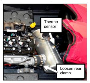
Step 15: Pull waterbox inlet out from exhaust coupler and remove waterbox from hull.
