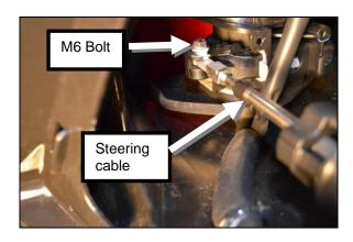
Step 6: Remove Torx screws (2) holding steering cable to top deck.
