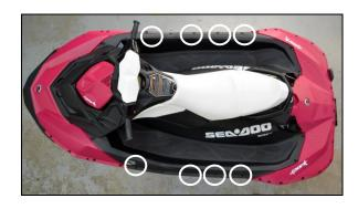
Step 26: Reinstall rear trim pieces (refer to step 8) & reinstall self tapping screws at front & back of hull. (circled in illustration below) Torque to 5.5 N.m / 49 inch lbs.
