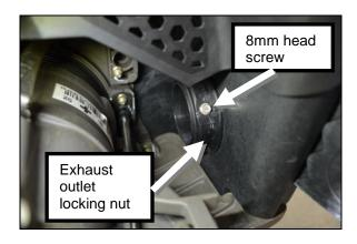
Step 12: Remove exhaust hose from waterbox & remove exhaust resonator box from hull.
