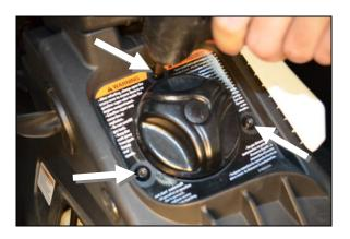
Step 9: With assistance, remove top deck by lifting straight up from lower deck. Guide steering cable through cable access hole in top deck.
