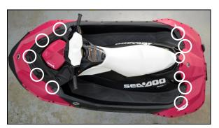
Step 27: Reinstall self taping screws (3) at gas fill cap. Torque to 4.5 N.m / 40 inch lbs. (refer to step 10)
