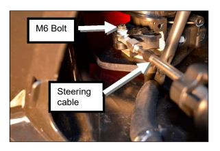
Step 6: Remove Torx screws (2) holding steering cable to top deck.
