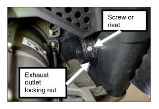
Step 14: Remove exhaust hose from waterbox & remove exhaust resonator box from hull.
