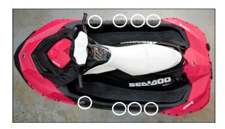
Step 24: Reinstall rear trim pieces (refer to step 8) & reinstall self-tapping screws at front & back of hull. (Circled in illustration below.) Torque to 5.5 Nm / 49 inch lbs.
