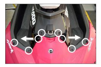
Step 9: Remove the ten (10) circled Torx screws & nuts on the sides of the hull. (See illustration below.)
