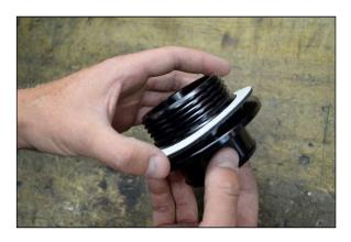
Step 16: Peel off backing on other side of rubber seal & install exhaust outlet from inside of hull. Install lock nut removed on step 13 onto billet exhaust outlet.
