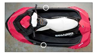
Step 22: Install rear support screws. (Circled in illustration below.) Torque to 5.5 Nm / 49 inch lbs.
