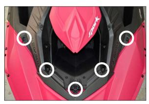
Step 8: Remove the eight (8) circled self-tapping screws at the rear of the top deck. Remove rear trim pieces by sliding out of position. (See illustration below.)
