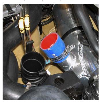
Thoroughly clean supercharger outlet and throttle body inlet using a non-residual cleaner. Reconnect and secure hoses to supercharger outlet and throttle body inlet. **NOTE: Do not over tighten clamps.**
