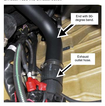
Ensure Free Flow Exhaust Tube is installed completely and secure hose clamps (3). **NOTE: Do not over tighten clamps.**
