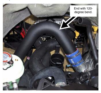
Thoroughly clean inside of exhaust outlet hose using a non-residual cleaner. Install opposite end of Free Flow Exhaust Tube into exhaust outlet.
