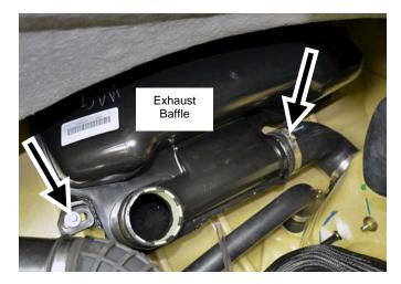
Remove bolt securing exhaust baffle to hull.
