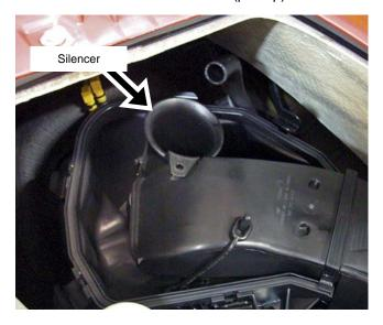
Remove rubber straps (3) securing air intake tube. Remove air intake tube. Set aside.
