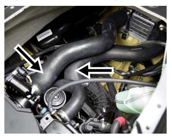
Loosen clamp securing exhaust outlet hose to exhaust baffle.
