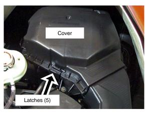
Lift cover and pull forward to gain access to blow-by hose. Remove hose. Set lid aside.
