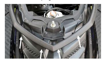
Remove bolt (1 at rear) and reusable clips (4 at front) securing decorative cover to outside of grab handle.
