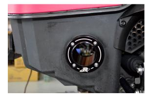
Step 19: Apply silicone to backside of retainer ring and install onto exhaust outlet from inside of hull. Secure exhaust outlet using supplied button head bolts. **Note:** Apply blue Loctite to threads of bolts. Do not overtighten bolts.
