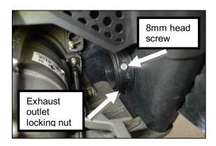
Step 14: Remove exhaust hose from waterbox & remove exhaust resonator box from hull.
