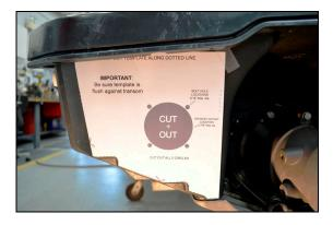
Outlet hole can be made using a hole saw bit, or with a Dremmel®, Roto Zip® or die grinder tool. Note: Start with a 2-3/4" hole saw bit. Wear safety glasses.
