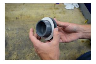
Step 16: Peel off backing on other side of rubber seal & install exhaust block off from inside of hull. Secure exhaust block off using lock nut removed in step 13.
