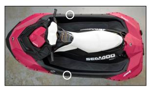
Step 26: Install rear support screws (circled in illustration below) Torque to 5.5 N.m / 49 inch lbs.
