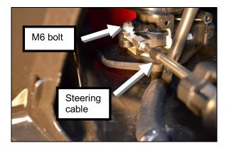
Step 6: Remove Torx screws (2) holding steering cable to top deck.
