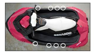
Step 28: Reinstall rear trim pieces & reinstall self tapping screws at front & back of hull. (circled in illustration below) Torque to 5.5 N.m / 49 inch lbs.
