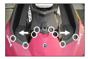
Step 9: Remove the ten (10) circled Torx bolts & nuts on the sides of the hull. (see illustration below)
