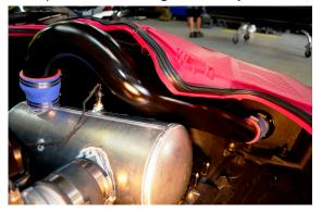
Step 24: Reinstall top deck to lower deck. (reference step 11) Make sure rear deck support is correctly positioned and top threaded inserts (2) are in place.
