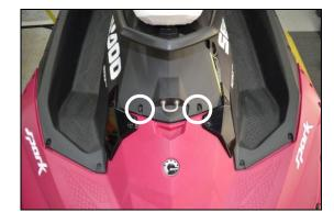
Step 27: Install side rail bolts, nuts & washers. (circled in illustration below) Torque to 3.5 N.m / 31 inch lbs.
