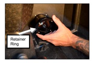
Step 20: Install 2.75" straight coupler to rear exhaust outlet. Apply glass cleaner to inside of coupler to ease installation. Secure using supplied #44 (larger) hose clamp. **Do not overtighten clamp.**
