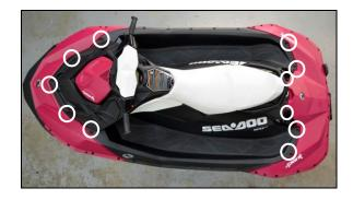
Step 29: Reinstall self taping screws (3) at gas fill cap. Torque to 4.5 N.m / 40 inch lbs.
