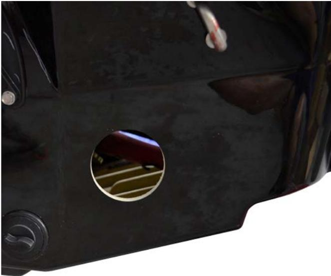
Install supplied billet exhaust outlet from outside and align so that 'R' logo is at bottom (6 o'clock). Drill bolt holes (4). Remove outlet. Thoroughly clean inside and outside of hull.
