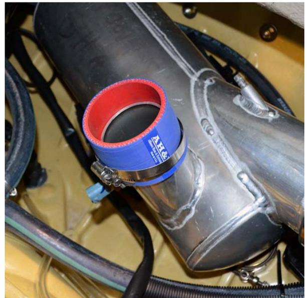
Install 4-1/2" long coupler onto long, straight end of supplied Rear Exhaust Tube. Secure using stock clamp.
