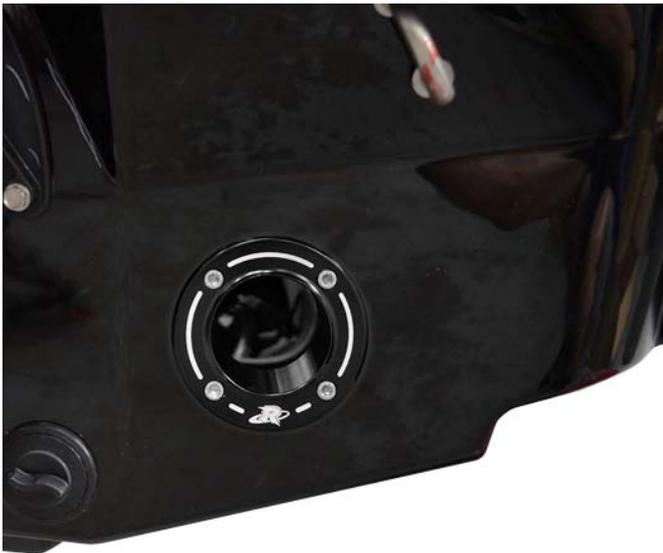
Install supplied rubber gasket onto Billet Exhaust Outlet flange. **NOTE: DO NOT APPLY SILICONE.**
