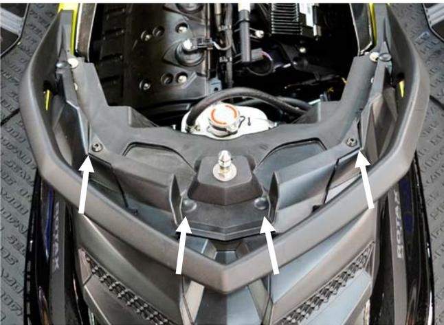
Remove bolt (1 at rear) and reusable clips (4 at front) securing decorative cover to outside of grab handle.
