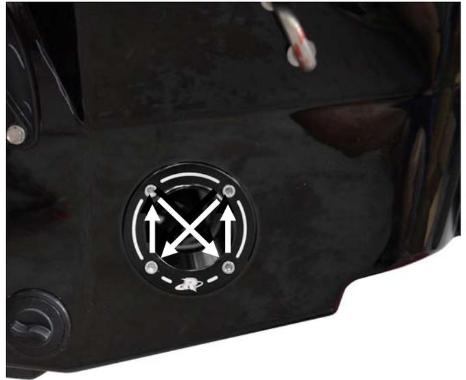
Secure using supplied bolts (4). **NOTE: Apply blue Loctite to bolts. DO NOT APPLY SILICONE.**
