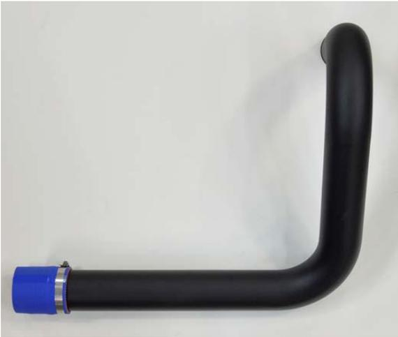
Place second clamp over coupler and tighten enough to hold in place.
