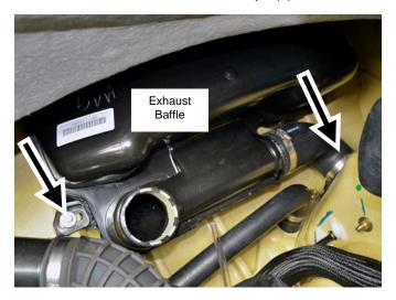
Install supplied block-off onto stock exhaust outlet. Secure with supplied clamp. **NOTE: Do not over tighten clamp.**
