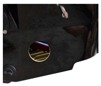
Install supplied billet exhaust outlet from outside and align so that 'R' logo is at bottom (6 o'clock). Drill bolt holes (4). Remove outlet. Thoroughly clean inside and outside of hull.
