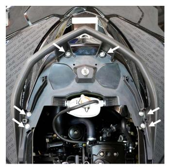
Remove exhaust hose between exhaust muffler (water box) and exhaust baffle. Retain clamps (2).
