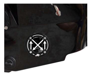
Secure using supplied bolts (4). **NOTE: Apply blue Loctite to bolts. DO NOT APPLY SILICONE.**
