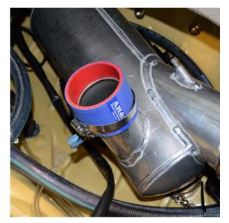
Install 4-1/2" long coupler onto long, straight end of supplied Rear Exhaust Tube. Secure using stock clamp. **NOTE: Do not over tighten clamp.**
