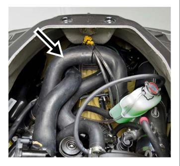
Remove hose between throttle body inlet and intercooler outlet.
