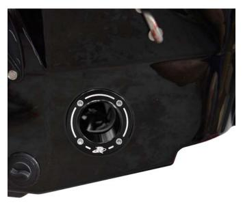
Install supplied rubber gasket onto Billet Exhaust Outlet flange. **NOTE: DO NOT APPLY SILICONE.**
