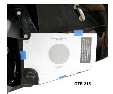
Mark hull at center of shaded circle (cross-hairs) using a punch or scribe.
