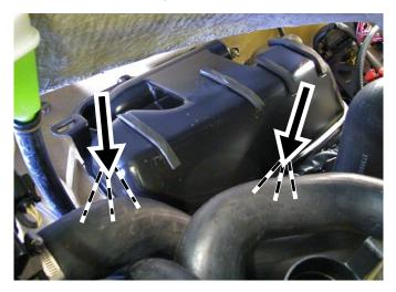
**TIP:** Spray glass cleaner onto hoses to make removal easier.
