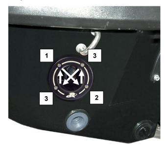
**WARNING:** Over tightening bolts will result in over compressing and distorting rubber gasket.
