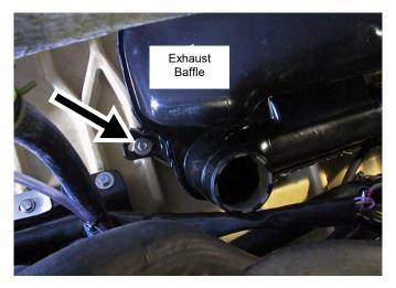
Pull exhaust baffle forward to remove from exhaust outlet. Twist baffle to flip over. Remove baffle.
