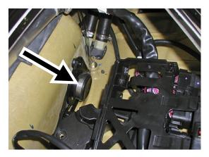
At rear of craft remove left deck hatch or storage bucket to access intercooler hoses.
