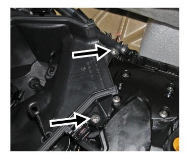
Squeeze outlet hose inside air intake silencer. Remove air intake silencer by lifting up. Set aside.
