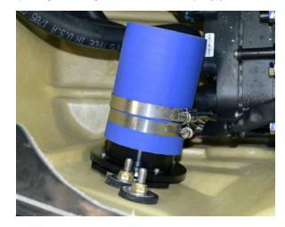
Install supplied rear exhaust tube straight end first from engine compartment. It will be necessary to twist as you "thread" the tube into place.
