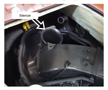
Remove rubber straps (3) securing air intake tube. Remove air intake tube. Set aside.
