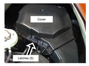
Lift cover and pull forward to gain access to blow-by hose. Remove hose. Set lid aside.
