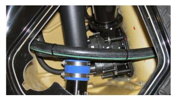
Secure clear syphon tubes (2) to top of Rear Exhaust Tube with remaining supplied zip tie.
