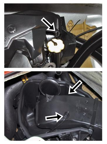
Remove bolts (2) securing air intake silencer to motor.
