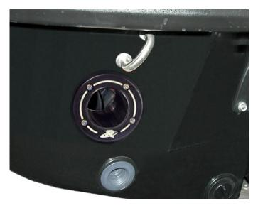
Install supplied rubber gasket onto billet exhaust outlet flange. NOTE: DO NOT APPLY SILICONE TO RUBBER GASKET.
