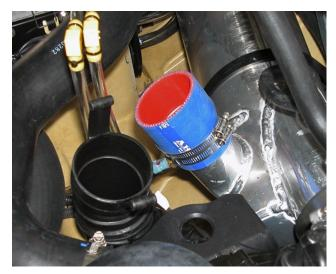
Install supplied coupler onto exhaust thru-hull outlet completely. Loosely install stock clamps (2).
