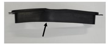
Clean cut edge of storage tub sealing flange.
