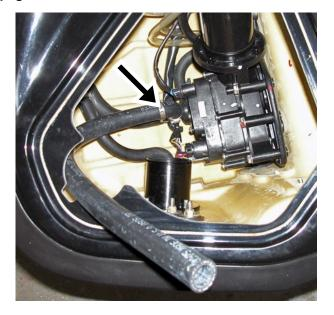
Thoroughly clean water box outlet with a non-residual cleaner. Install supplied coupler onto water box outlet completely. Secure using stock clamp. **NOTE: Do not over tighten clamp.** Loosely install second stock clamp over coupler.
