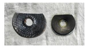
Replace washers with flat side facing downward towards bottom of craft. Secure with stock nut. **NOTE: Do not over tighten nut.**
