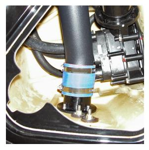
Ensure exhaust tube is properly aligned and curved end of exhaust tube is flush against water box outlet. Tighten all clamps. **NOTE: Do not over tighten clamps.**
