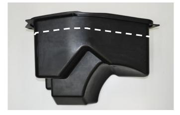
Cut off bottom of storage tub. **TIP:** Use a large gate band saw if available. Place a thin piece of wood under right side of sealing flange  $(1/2^{\circ} - 3/4^{\circ})$  thick).
