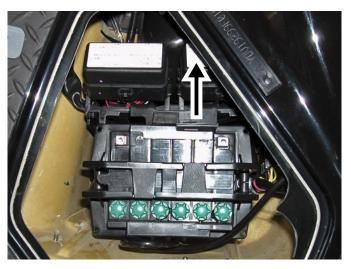
Remove bolts (2) securing battery holder to hull. Remove battery holder.
