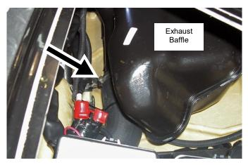
Remove exhaust hose between exhaust muffler (water box) and exhaust baffle. Retain hose clamps (2).
