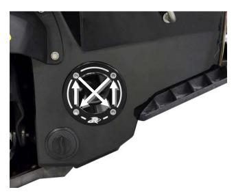
Secure using supplied bolts (4). **NOTE: Apply blue Loctite to bolts. NOTE: DO NOT APPLY SILICONE.**
