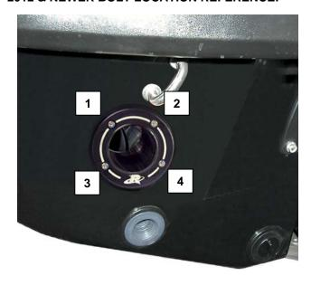
Secure outlet using supplied bolts (4). **NOTE: Apply blue Loctite to bolts. Do not over tighten bolts.**
