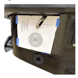
Mark hull at center of shaded circle (cross-hairs) using a punch or scribe.
