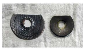
Replace washers with flat side facing downward towards bottom of craft. Secure with stock nut. **NOTE: Do not over tighten nut.**
