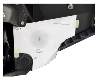
Mark hull at center of shaded circle (cross-hairs) using a punch or scribe.
