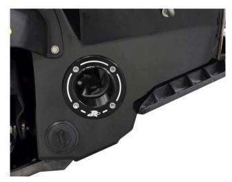
Install supplied rubber gasket onto Billet Exhaust Outlet flange. **NOTE: DO NOT APPLY SILICONE**.
