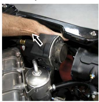
Allow tail section of exhaust to relax. Apply red Loctite to exhaust bolts (4). Loosely install into exhaust tail section, but do not thread into exhaust pipe.
