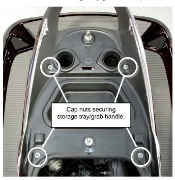
**TIP:** Replace cap nuts on studs for storage tray to prevent injury while performing work.
