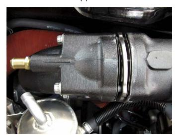
Slide water box strap backwards on top of water box.
