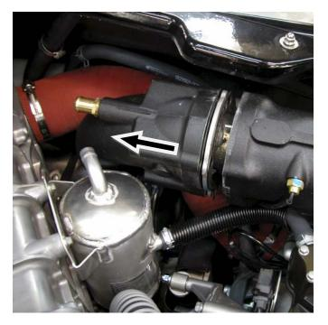
Pull back and up on exhaust tail section to remove Exhaust Filter with gaskets.
