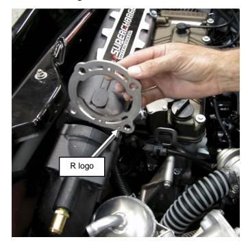
While holding Exhaust Race Plate and gaskets in place thread bolts into exhaust pipe 4~5 times.
