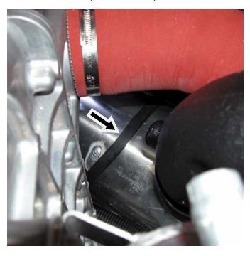
Move water box and exhaust tail section backwards as far as it will go. **NOTE: Make sure Exhaust Filter and Gaskets move with exhaust tail section.**
