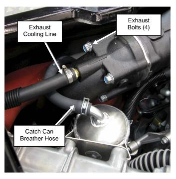
Remove bolts (4) securing exhaust tail section to exhaust pipe.
