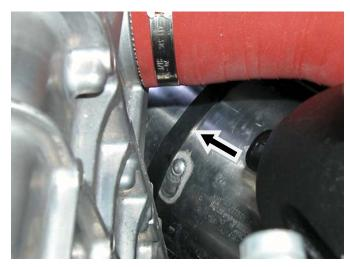
Move water box and exhaust tail section forward to join exhaust tail section with exhaust pipe. Tighten bolts in a criss-crossing pattern. **NOTE: Torque bolts to 33 ft•lb / 45 N•m.**
