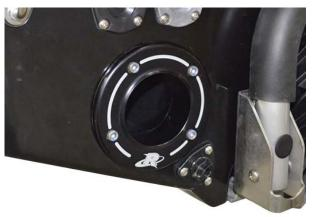
Inside hull place one stock clamp (loosely) over exhaust outlet coupler.
