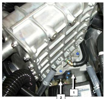
Remove bolts<sup>2</sup> (2) securing intercooler to hull.
