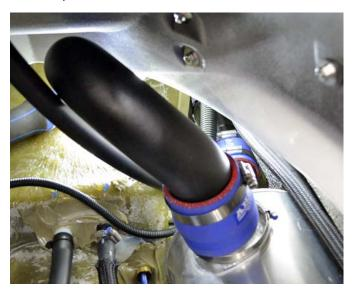
Secure coupler to water box outlet. **NOTE: Do not over tighten clamp.**
