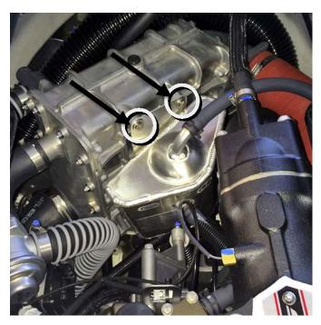
Disconnect hoses attached to oil separator tank and remove tank from engine compartment.
