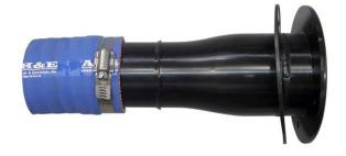
Install Billet Exhaust Outlet into hull and secure using stock hardware. NOTE: Be sure rubber gasket is in place between flange and hull. Do not apply sealant to gasket. Apply blue Loctite to bolts. Do not over tighten bolts.
