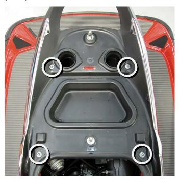
**TIP:** Cover the four studs for storage tray with several pieces of tape to prevent injury while performing work.
