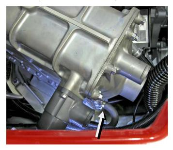
Remove intercooler by rotating air outlet side upward while lifting.
