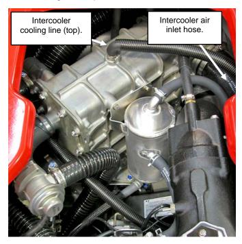
**2008~2010 models only:** Disconnect cooling line secured to top of intercooler.
