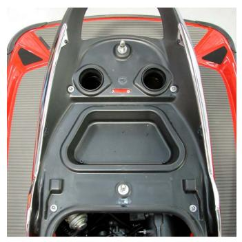
**TIP:** Replace cap nuts on studs for storage tray to prevent injury while performing work.
