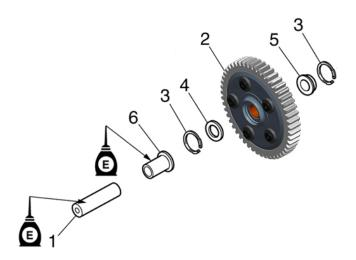
IMPORTANT: Note orientation of Supercharger Gear Dampener and it's components as you assemble.
