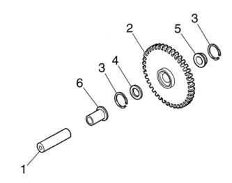
IMPORTANT: Note orientation of idler gear and it's components as you disassemble.
