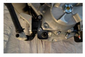
Remove the 14mm head exhaust pipe mounting bolt.
