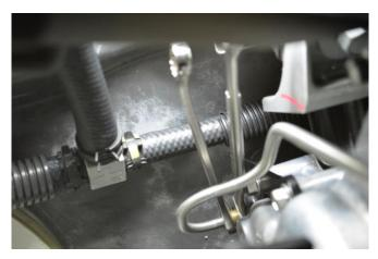
Tighten the 14mm head exhaust mounting bolt holding the upper oil tube bracket in place. Torque bolt to 31 foot pounds.
