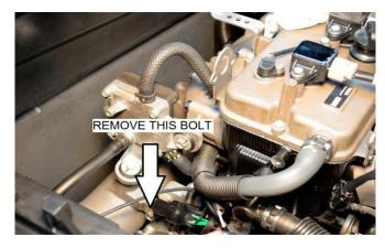
Place the oil extraction tube in position by fastening the upper mounting bracket in place using the 14mm head exhaust pipe mounting bolt. Do not tighten, keep very loose.
