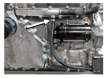
Secure cooling lines together using supplied zip tie.
