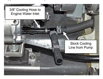
Route 3/8" line forward under engine and up towards exhaust manifold. Attach open end to fitting on engine water inlet. Secure using supplied 1/2" hose clamp.
