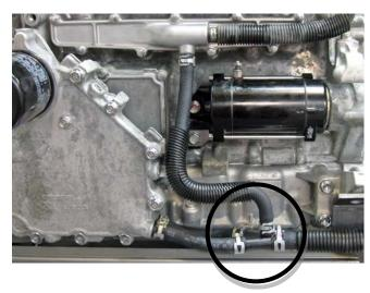
Disconnect lines attached to both ends of 'Y' fiting (1 incoming / 2 out to oil cooler). Disconnect cooling line attached to engine water inlet fitting.
