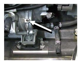
Reconnect exhaust outlet tube to waterbox outlet coupler. Once aligned tighten coupler clamps (inlet and outlet). **NOTE: Do not over tighten clamps.**
