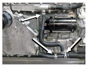
Remove 'Y' fitting with line for engine water inlet and discard.
