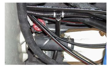
Route 1/2" cooling line through opening in bulkhead for exhaust.
