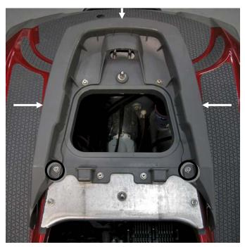
Remove strap securing waterbox in place. Loosen coupler clamp and remove exhaust outlet tube.
