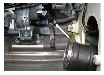
Remove 'T' fitting with lines (2) attached.
