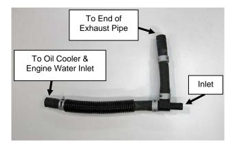
Remove cooling line for end of exhaust pipe from plastic 'T' and install onto supplied billet 'T' fitting in same configuration. Secure with stock spring clamp. Install supplied 3/8" cooling line onto 3/8" barb of 'T' fitting and secure with supplied 1/2" hose clamp. **NOTE: Do not over tighten clamp.**
