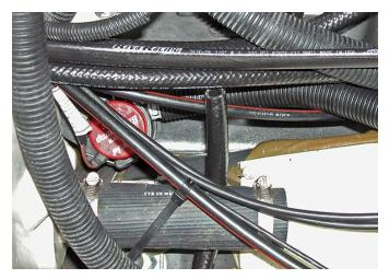
Splice the intercooler cooling line and install the supplied 1/2" 'T' fitting. Install the supplied 1/2" line onto 'T' fitting. Secure lines using supplied 3/4" hose clamps.
