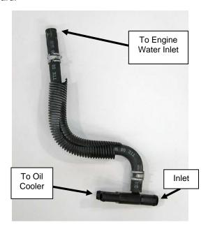
At rear of same side of engine disconnect the line feeding plastic 'T' fitting.
