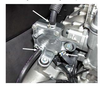
Remove bolt securing end of exhaust pipe to motor. Disconnect exhaust pipe overheat sensor connector (green). Disconnect cooling line from underside of end of exhaust pipe. Loosen clamp securing coupler to end of exhaust pipe.
