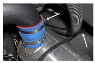
Remove engine breather line(s) from engine breather box.
