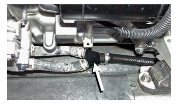
Install supplied billet 'T' fitting into stock cooling line from pump and secure with stock spring clamp.
