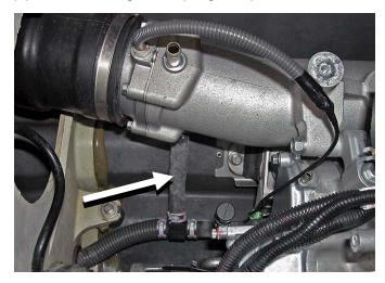
Replace bolt securing end of exhaust pipe to motor.
