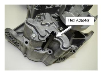
Using a 13mm socket, tighten the black hex adaptor piece to 5 foot pounds. (60 inch pounds) **DO NOT OVERTIGHTEN THE HEX ADAPTOR!** Over tightening the hex piece may result in the threads breaking off in the oil pump.
