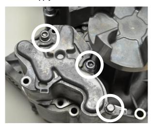
Do not fully tighten bolts yet. Keep cover plate slightly loose. Make sure the new o-ring is secure in the o-ring groove & does not get pinched or damaged.
