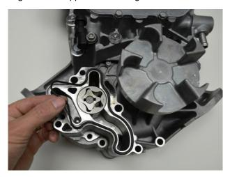
**Tip:** Apply grease to the new o-ring before installation. This will assist with holding the o-ring in place when reinstalling the oil pump cover.
