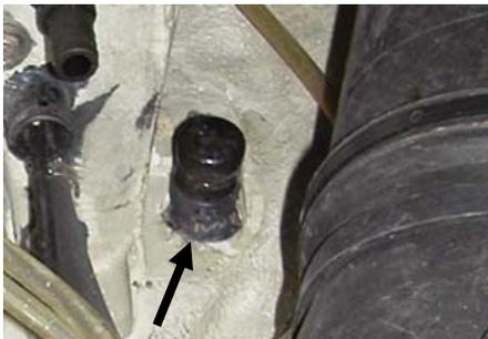
Install supplied sacrificial zinc anode into supplied Billet Water Pump Cover.
