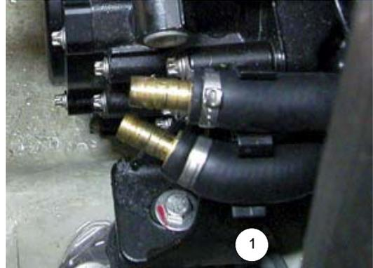
**NOTE: Install larger end of splicer into oil cooler hose.**
