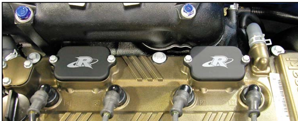
Valve Cover Block-off's installed.
