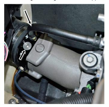
Install supplied stainless O2 sensor block-off fitting with crush washer. **NOTE: Apply Loctite 518 to threads. Torque to 28 ft-lb / 38 N-m.**
