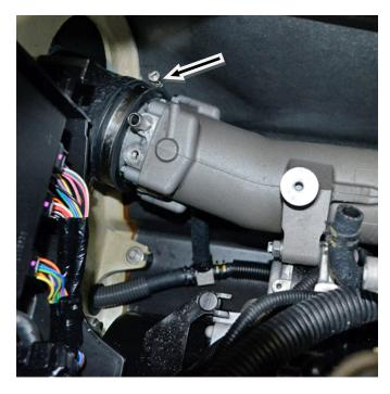
Remove bolts (11 total) securing exhaust pipe assembly to motor.
