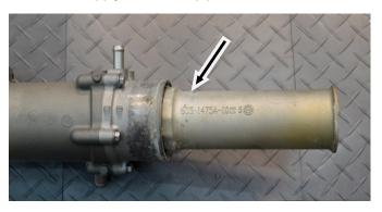
Using the Yamaha Exhaust Pipe Wrench part# YW-06726 (90890-06726-00) and a large breaker bar remove tail pipe extension. **CAUTION: Tail pipe will be extremely hot. Wear protective gloves when handling tail pipe extension.**
