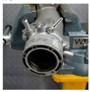
Install supplied billet tail pipe with stock tail pipe gasket. NOTE: NOTE: If exhaust gaskets are damaged, warped or corroded do not reuse. Apply blue Loctite to bolts. Torque in criss-cross sequence: 1st 11 ft•lb / 20N•m; 2nd 21 ft•lb / 29N•m
