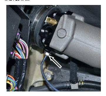
Connect cooling line from regulator/rectifier to tail pipe.
