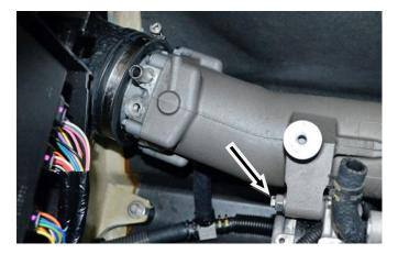
Rotate exhaust pipe assembly away from motor towards hull. Disconnect cooling line at underside of tail pipe.
