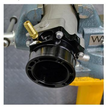
Install and secure tail pipe extension. NOTE: Apply Loctite 648 to threads. Torque to 46 ft•lb / 63 N•m.
