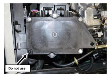
Replace relay box onto electrical box backing plate using one original bolt. At opposite side use supplied M6 bolt, washer and spacer to secure relay box to electrical box. NOTE: Apply blue Loctite to threads. Do not over tighten bolts.
