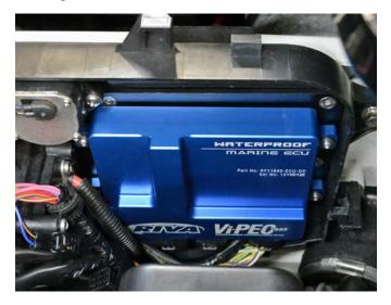
Secure wiring harness at lower, right side of electrical box using supplied zip tie.
