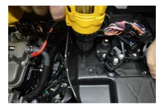
Rotate relay bracket in position & secure with supplied M6 bolt, spacer, washers (2) and nylon lock nut. Tighten both relay bracket bolts.
