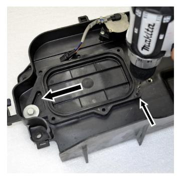
Locate and drill 1/4" hole through electrical box backing plate.
