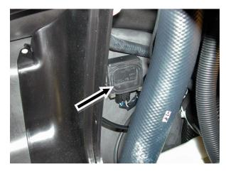
Disconnect electrical connector and install supplied block-off into wiring harness connector. **NOTE: Make sure block-off 'snaps' into place.**
