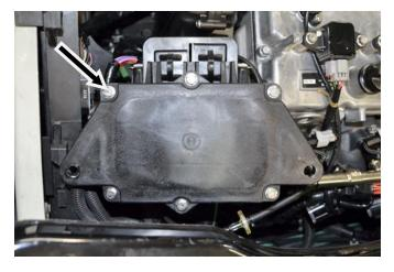
Remove electrical box backing plate from hull and set aside.
