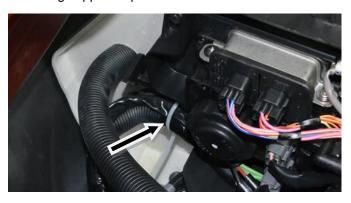
Replace electrical box cover. Carefully slide into place so that wiring harnesses fit into cut out.
