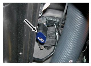
**NOTE:** If a RIVA/Vi-PEC V88 ECU was previously installed you must swap the black block-off with the supplied blue block-off.
