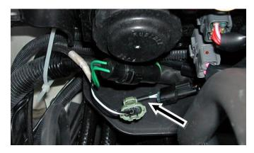
Connect stock ECU connectors (3) to Vi-PEC V88R3 ECU. **NOTE: Do not force. Verify order, location, and orientation. Listen/feel for click when locked in place.**
