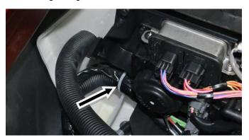
Follow harness and locate crank sensor connector. (black & white wire/black plug) Install supplied cable splicer between connectors for black & white wiring harness.
