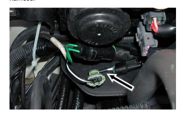
Connect stock ECU connectors (3) to Vi-PEC V88R3 ECU. **NOTE: Do not force. Verify order, location, and orientation. Listen/feel for click when locked in place.**
