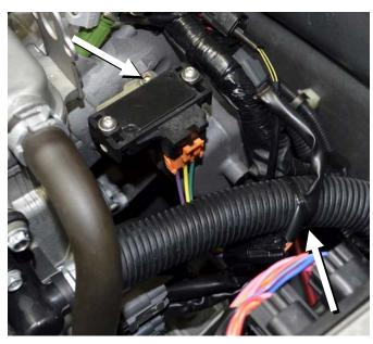
Connect open end of map sensor wire to wiring harness. Secure to cooling hose using supplied large zip tie.
