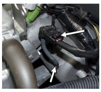
Under map sensor disconnect vacuum hose from intake manifold.
