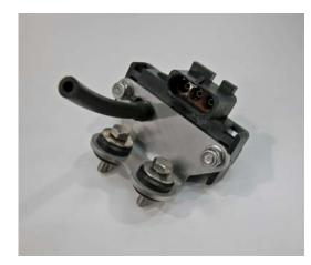
Install 3 Bar Map Sensor onto intake manifold.
