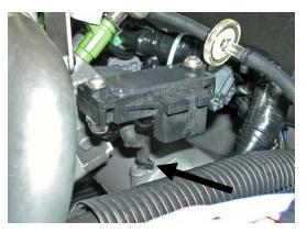
Attach orange end of supplied connecting coupler to 3 Bar Map Sensor. Attach opposite end to stock map sensor connector.
