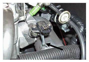
Remove bolts (2) securing map sensor bracket to intake manifold. Remove stock map sensor.
