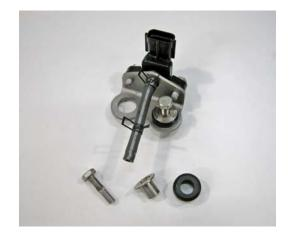
Install rubber collars, grommets and bolts into bracket on supplied 3 Bar Map Sensor.
