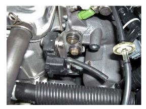
TIP: Install bolt closest to engine first with 3 Bar Map Sensor rotated upwards to allow access to underside. When snug rotate down to level and install second bolt. NOTE: Apply blue Loc-tite to bolts. Torque bolts to 3.7 lbf•in / 5 N•m.
