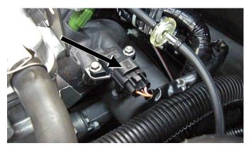
Under map sensor disconnect vacuum hose from intake manifold.
