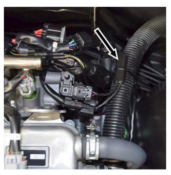
Secure map sensor to large hose using supplied zip tie.
