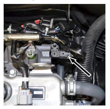
Install supplied Boost Clamp between stock map sensor and electrical connector.
