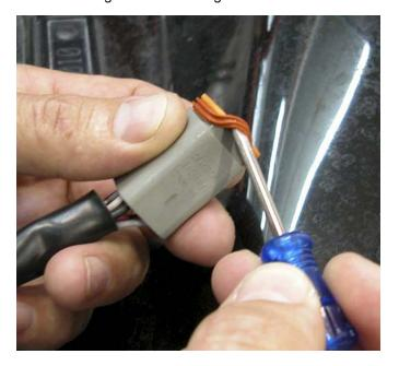
Carefully pry up edge of connector cap to remove.
