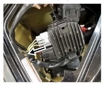
Follow voltage regulator wiring harness from connectors back to fuse boxes.
