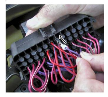
Flip fuse box over to view fuses. Install fuse (supplied item #3) into fuse panel across locations 'E6 & E7'.
