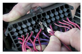
Insert one end of Jumper Wire (supplied item #5 – medium gauge red with blue stripe wire) into location 'C6'. (Listen for a click!) Pull back on wire to ensure terminal is locked in place.
