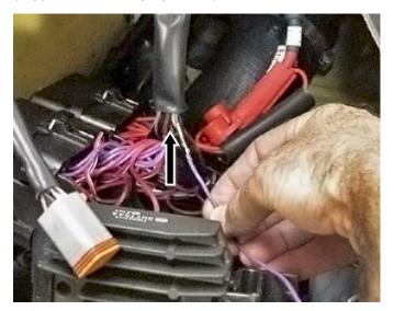
Feed purple wire into and through first section of sheathing to voltage regulator connectors. Pull purple wire through first section of sheathing. Insert and feed into second section of sheathing until end reaches diagnostic connector.
