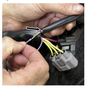
Remove o-ring from end of diagnostic connector.
