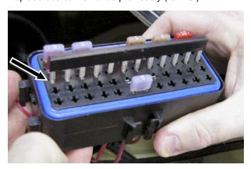
NOTE: It is important that you press bus bar evenly into place and straight down. Do not work side to side or bend pins.
