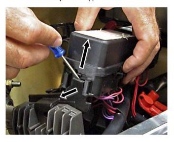
Remove fuse box cover to access fuses and bus bar.
