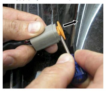
Remove white plastic plug (block-off) from pin hole #6.
