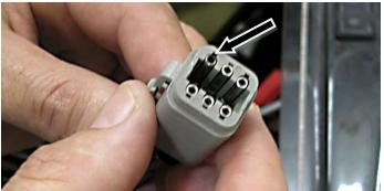
Replace connector cap and o-ring.
