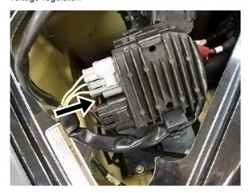
Rotate electrical component support to access fuse boxes. Remove fuse box closest to voltage regulator from electrical component support.
