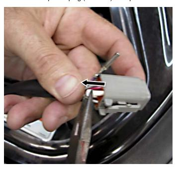
Insert end of Electrical Harness Wire (purple wire) into connector and lock into place. (Listen for a click!) Pull back on wire to ensure terminal is locked in place.
