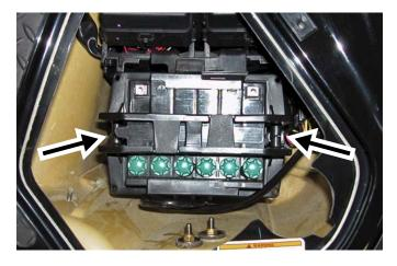
Align Speed Control Override Module (supplied item #1) with negative side of battery holder. Drill holes (2) for mounting hardware.
