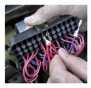
Insert end of Electrical Harness Wire (supplied item #4 – small gauge purple wire) into location 'E6'. (Listen for a click!) Pull back on wire to ensure terminal is locked in place.
