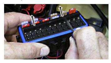
Remove rubber seal plugs from locations 'D6, D7, D8, E6 & E7' by pressing a small screwdriver into openings on top of fuse box. Seals will pop out at underside.
