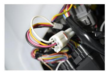
Push down lock tab on connector & disconnect plug.
