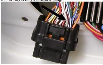
Secure wires in plug by depressing white tabs (2) below connector locking tab. You will hear a "click" when they are fully locked in position. Make sure both tabs are flush with the connector plug.
