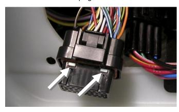
NOTE: Tabs must be pressed in evenly. Ensure all wires are installed in connector properly.
