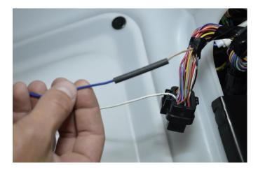
Using a heat gun, carefully warm up heat shrink tube until it collapses around wires. **NOTE: Do not use high heat or hold in one place. Move heat gun around continuously.**
