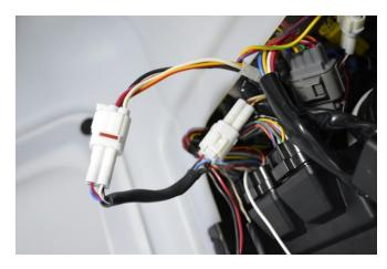
Reconnect black ECU plug into ECU. Ensure plug is fully installed & tab is locked.
