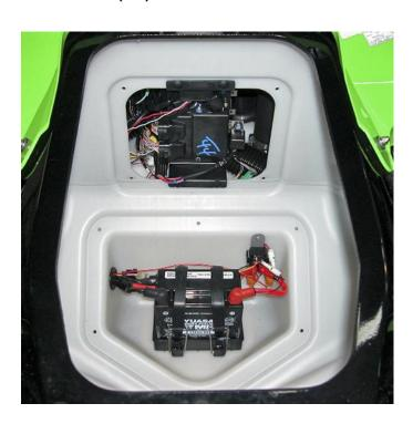
Remove adhesive backing from Dual Lock. Affix S.C.O.M. unit to underside of ECU bracket at top. (see next illustration)
