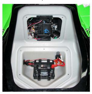
Remove adhesive backing from Dual Lock. Affix S.C.O.M. unit to underside of ECU bracket at top.
